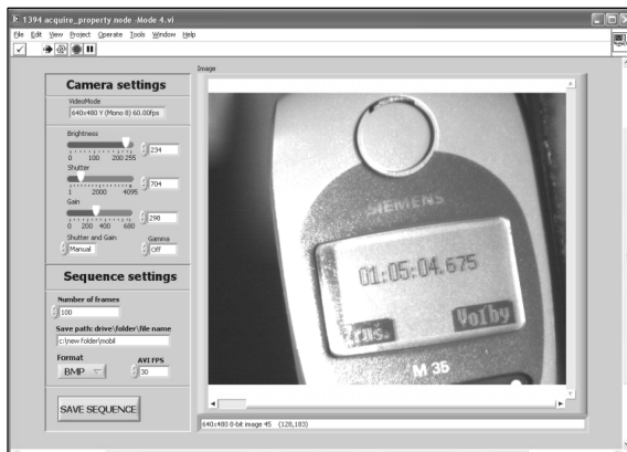
Obr. 4 Front Panel skriptu na záznam sekvencie Fig. 4 Front Panel of script for frequency acquire
